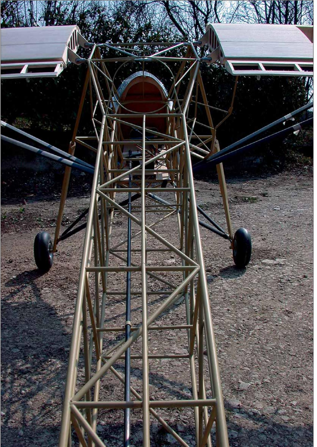
end I handed the fuselage to my friend Perfetto (modeller and car body repairer), who sprayed it with a layer of primer. Looking at it with that ochre colour looked like the fuselage of a real plane.
