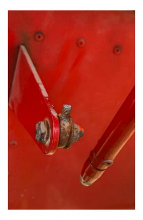
Its mandatory to do the daily inspection checks, control all movable parts on control surfaces for rust or oxidation. Grease all parts necessary to be greased and pay special attention to uniballs, those has to be greased with adequate grease or lube. The uniball has to be greased not only outside but mainly inside as shown on the picture
